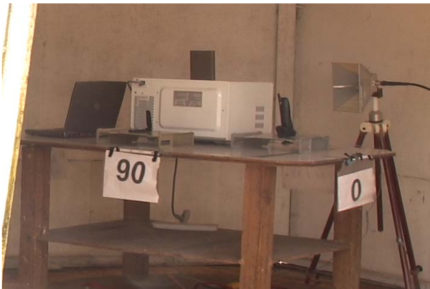
6. Cordless Phone, Microwave Oven and Laptop test setup, Large Bioprotector product present.
