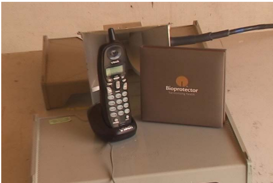
4. Cordless Phone test setup, Large Bioprotector product present.
