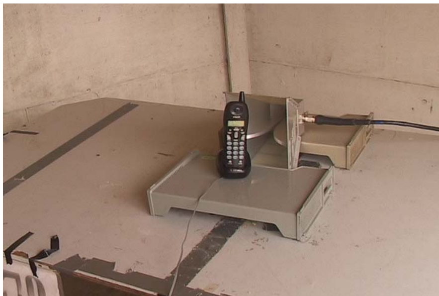
2. Cordless Phone test setup, no Bioprotector product present.
